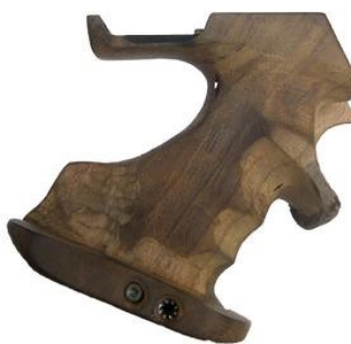
The hand support base copied and secured with two screws
