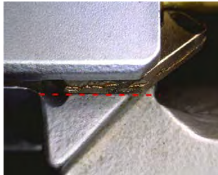
Extractor with fired case (bolt open)
