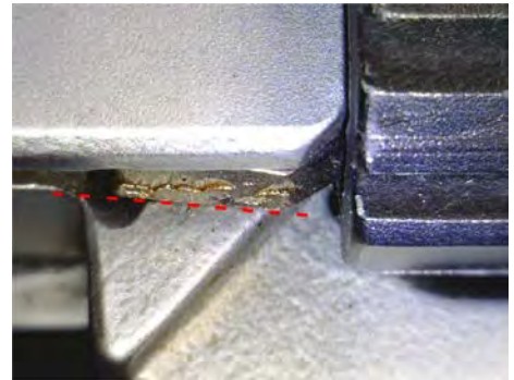
Extractor deflected by barrel slot
