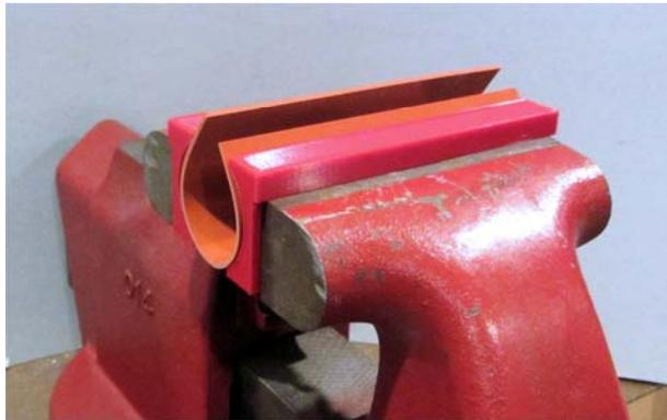
Insert the cylinder, tighten the vise good & snug, install the spanner and heave...
