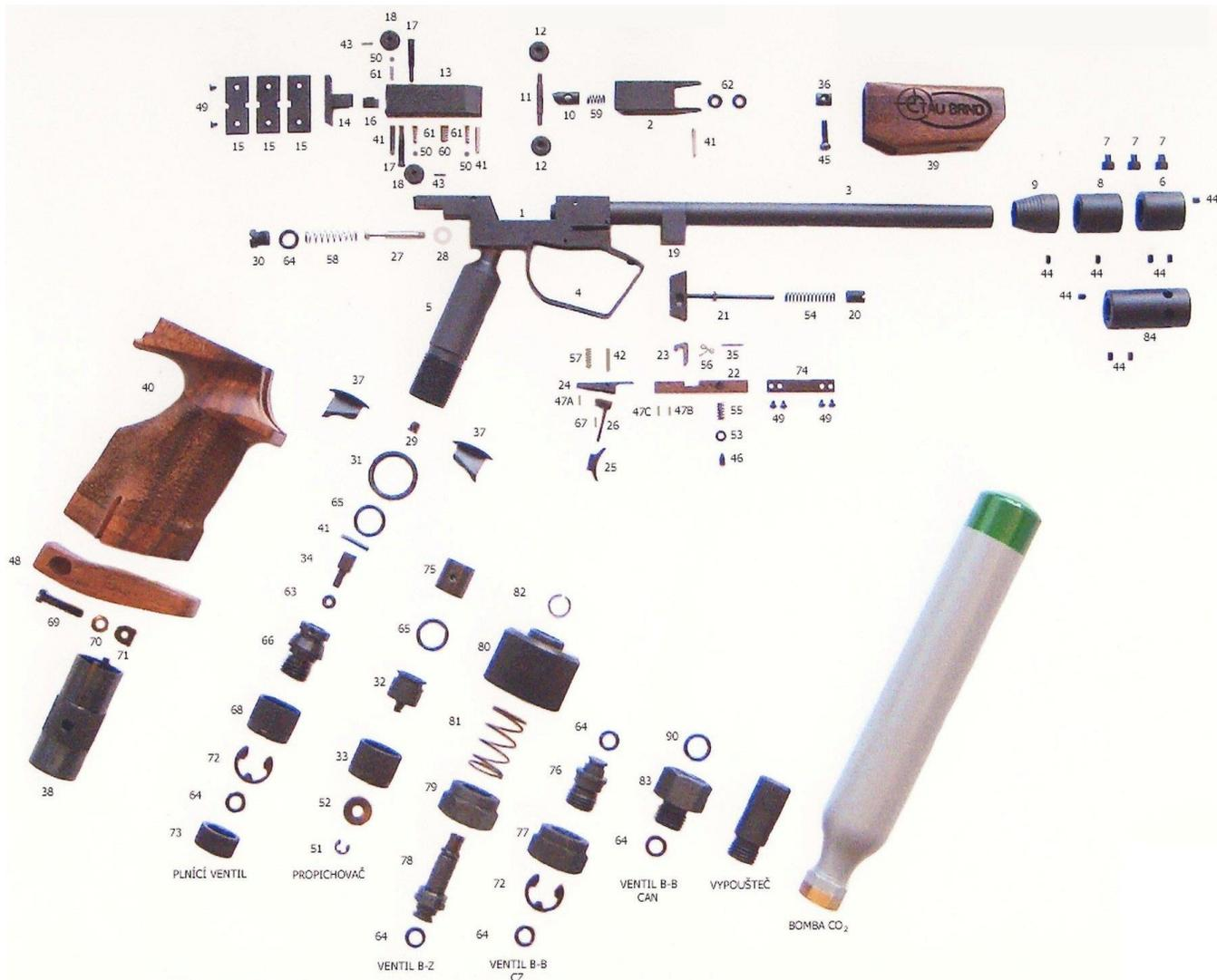
Some of this should be used with caution, because BRNO has made some design changes over the years. For example, very early diagrams show a #63 O-ring used as a seal for a small plug in the bottom of the frame in the trigger area. This feature is entirely absent in the picture above, and I don't think I've ever actually seen a pistol that has one. Here's a list of the O-ring part numbers & what they are used for:
