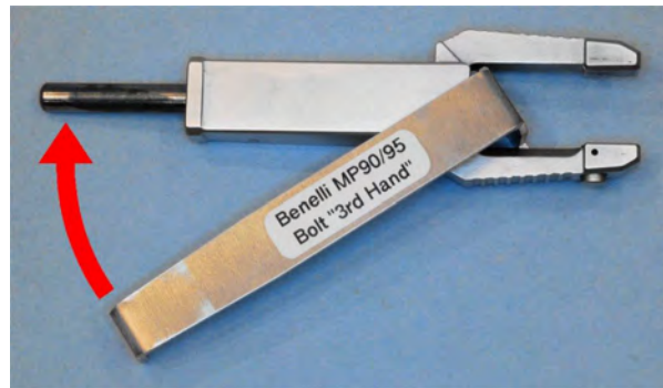
Figure 4: Installing bolt tool, Step 2
